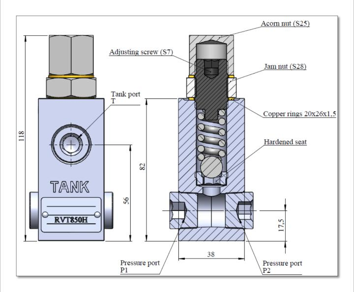
To adjust relief please remove acorn nut loosen jam nut, turn the adjusting screw clockwise to increase the pressure and counterclockwise to decrease the pressure.
