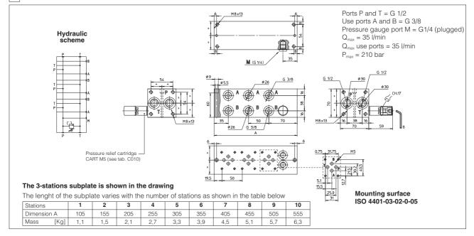
7 OVERALL DIMENSIONS OF SUBPLATES TYPE BA-214/\*/MH/\*-AL [mm]
