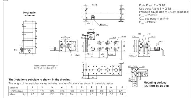
(1) The venting directional valve in the dashing line must be ordered separately
