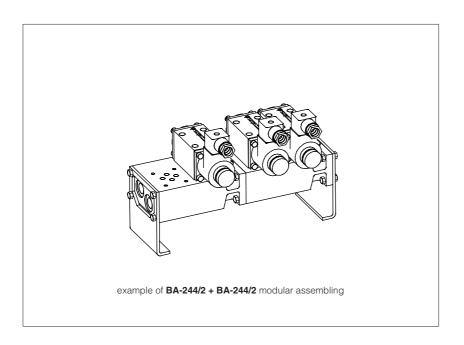
**BA-244** are **modular subplates** with 1 to 4 stations for valves ISO 4401 size 06. They are designed for installation on
