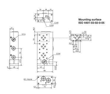
Fastening bolts: 4 exagonal head screws M6x20 class 12.9 included in the supply Tightening torque = 15 Nm Seals: 2 OR-3081 included in the supply
