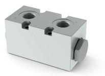
CM3P type modular check bankable valves allow one way free flow by raising a conical shutter, while in the opposite direction the fluid can return by means of a small piston piloted by the pressure in the other line.
