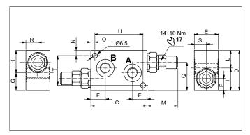
The direct acting compensator valves with CMP04 type cartridge protects the hydraulic components from impact or peaks in pressure.
