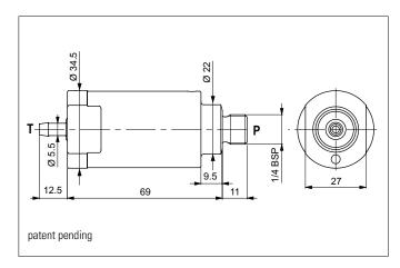
Valve used on power units to generat a flow rate ramp on the actuator to delay system pressurisation and allow the single phase motor to reach the required speed.
