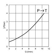
Fluid used: mineral based oil with viscosity 32 mm<sup>2</sup>/s at 40°C.
