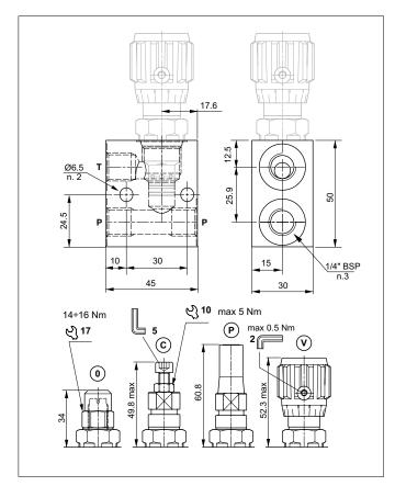
The direct acting relief valve with CMP04 cartridge limits the pressure in the hydraulic circuit
