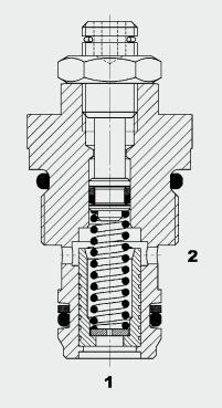
The SR5E is a pressure compensated flow control valve which maintains a constant outlet flow by means of a control function. The flow rate is largely independent of the pressure and viscosity.
