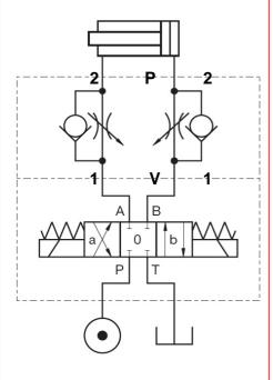
Needle Valve with reverse flow check Sandwich plate type ZW-SDR10
