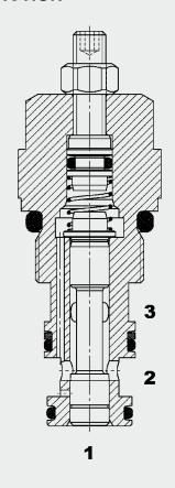
The SDH05330 is a hydraulically operated, spring-loaded, adjustable spool valve. In the normal position, the valve is open and there is flow from port 3 to port 2. When control pressure is applied to port 1, the valve switches into the flow control position and the flow is reduced.
