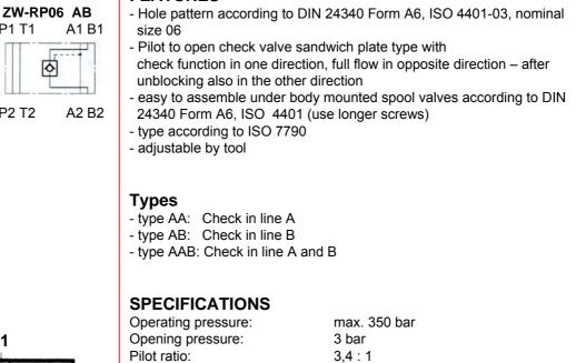
max. 50 l/min (in controlled lines) max. 75 l/min (in free lines) hydraulic oil according to DIN 51524 Part 1 and 2 Media operating temp. range: -20°C up to max. +80°C Ambient temperature range: -20°C up to max. +50°C 10 - 400 mm<sup>2</sup>/s is recommended Class 20/18/15 to ISO 4406 or cleaner 1,3 kg incl. Valves
