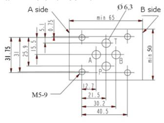
Mounting screws: M5 x 30 DIN 912-10.9
