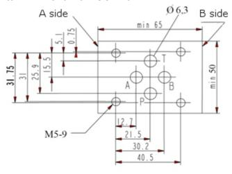
Mounting screws: M5 x 30 DIN 912-10.9
