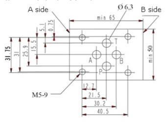
Mounting screws: M5 x 30 DIN 912-10.9
