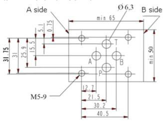
Mounting screws: M5 x 30 DIN 912-10.9
