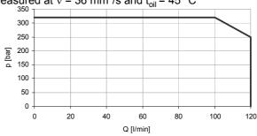
The operating limits were determined using coils at operating temperature and 10% under voltage. The operating limits given are for applications with two flow directions. For flow in only one direction, the operating limits can be lower.
