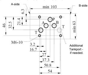
Mounting screws: M6 x 40 DIN 912-10.9
