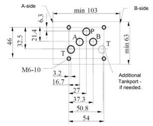
Mounting screws: M6 x 40 DIN 912-10.9
