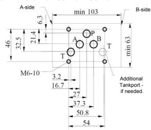
Mounting screws: M6 x 40 DIN 912-10.9
