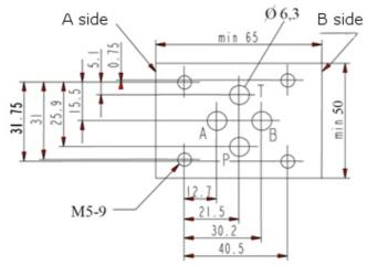
Mounting screws: M5 x 30 DIN 912-10.9
