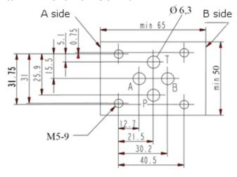
Mounting screws: M5 x 30 DIN 912-10.9
