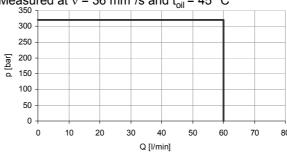
The operating limits were determined using coils at operating temperature and 10% under voltage. The operating limits given are for applications with two flow directions. For flow in only one direction, the operating limits can be lower.
