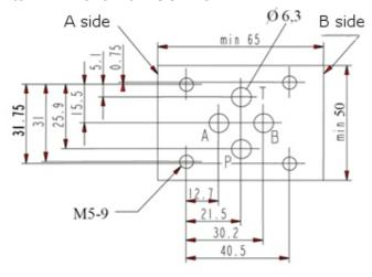
Mounting screws: M5 x 30 DIN 912-10.9
