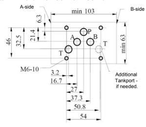
Mounting screws: M6 x 40 DIN 912-10.9
