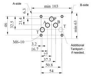
Mounting screws: M6 x 40 DIN 912-10.9
