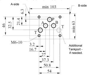
Mounting screws: M6 x 40 DIN 912-10.9
