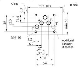
Mounting screws: M6 x 40 DIN 912-10.9
