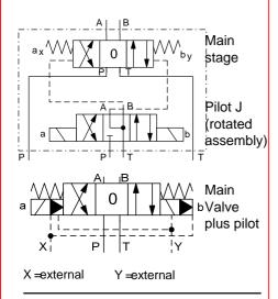
4/2 directional valve with spring offset Type 4WEH 10, 16
