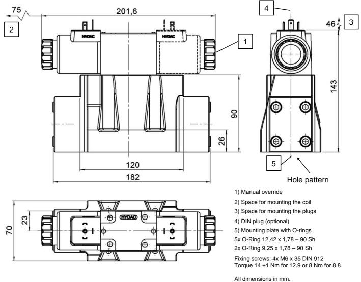
Fixing elements are not in the scope of supply .
