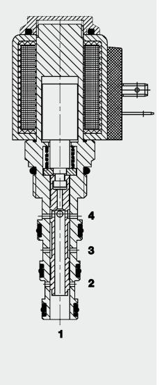
When the solenoid coil is de-energized, there is flow through the valve from port 4 to port 1. Ports 2 and 3 are closed. When the solenoid coil is energized, there is free flow through the valve from port 3 to 4 or from 4 to 3 and also from port 2 to 1 or from 1 to 2. **4/2 Solenoid Directional Valve UNE Spool Type - Direct-Acting SAE-08 Cartridge – 350 bar** WK08P-01
