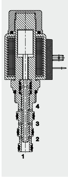
When the solenoid coil is not energized, there is free flow through the valve from port 3 to 4 or from 4 to 3 and also from port 2 to 1 or from 1 to 2. In the energized mode, the valve blocks
