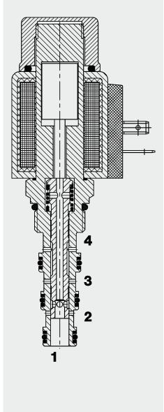
When the solenoid coil is de-energized, all ports are closed. When the solenoid coil is energized, there is free flow through the valve from port 1 to 2 or from 2 to 1 and also from port 3 to 4 or from 4 to 3. **4/2 Solenoid Directional Valve UNE Spool Type, Direct-Acting SAE-08 Cartridge – 350 bar** WK08Z-01
