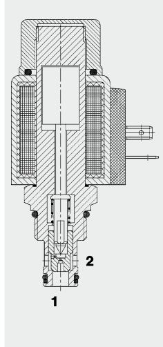
When de-energized, there is free flow through the valve from port 2 to port 1. Flow is not possible in the reverse direction.
