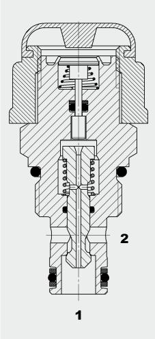
The directional valve WS08W...M is a normally closed, manually operated poppet valve.
