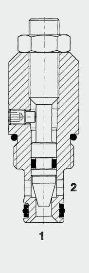
The SD08 is a flow restrictor valve which controls the flow rate by means of an adjustable cross section. The flow rate is therefore dependent on the pressure differential and viscosity. Starting with the throttle spindle in the fully closed position, the flow rate increases in accordance with the appropriate curve as the control knob is turned. The flow is controlled in both directions. Needle Valve SAE-8 Cartridge – 420 bar SD08-01
