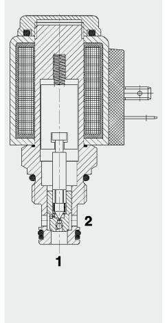
2/2 Solenoid Directional Valve Poppet Type, Pilot Operated Normally Closed (Reverse Flow) Metric Cartridge Valve – 350 bar
