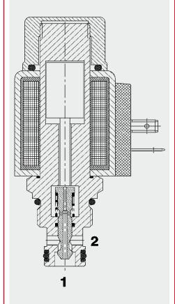
When the solenoid coil is de-energized, the valve blocks flow in both directions. When energized the valve allows flow in both directions.
