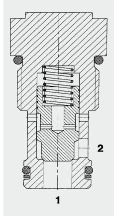
The check valve RV12A-01 is a direct acting cone poppet type valve which allows flow in one direction and shuts off flow in the opposite direction. When there is no flow through the valve, the spring holds the poppet in the closed position and therefore shuts off port 2 from port 1. The valve opens when the pressure at port 1 is higher than the pressure at port 2, including the pressure created by the spring force.
