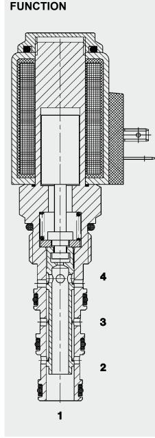
When the solenoid coil is de-energised, the valve allows flow in both directions between ports 3 and 2 and in both directions between ports 4 and 1. When the solenoid coil is energized is free flow through the valve directions between ports 3 a also between ports 1 and 2. the solenoid coil is energized, there is free flow through the valve in both directions between ports 3 and 4 and
