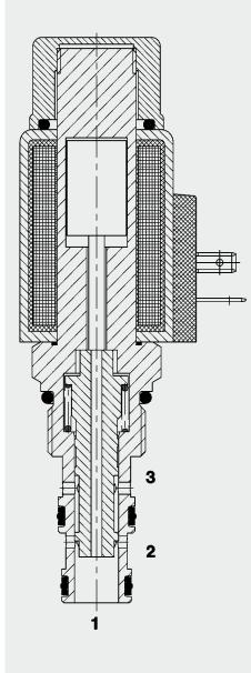
When the solenoid coil is de-energized, the valve allows flow in both directions between ports 2 and 1, while blocking
