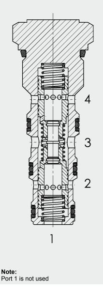
The ST10 flow divider is a spring-loaded pressure compensated spool type valve. It divides a flow in two and keeps both flows constant. The division is made according to the specified ratio - from port 3 to ports 2 and 4. As a flow combiner it combines two
