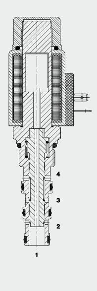
When de-energized, the valve allows flow in both directions between ports 1 and 2. When the solenoid coil is energized valve is closed in both directions. flow in both directions between ports 3 and 4 and also in both directions
