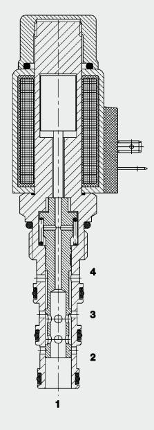
When de-energized, the valve allows flow from port 3 to 1 or from 1 to 3, while blocking flow at ports 2 and 4. When energized, the valve allows flow
