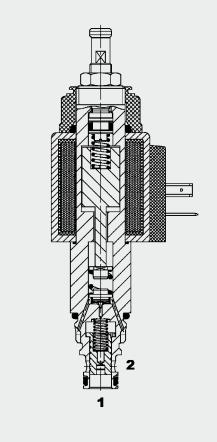
The PDB08PZ is a pilot-operated, spool type proportional pressure relief valve. If pressure at port 1 exceeds the setting defined by the electrical signal, the pilot poppet opens and oil flows from behind the main spool to tank port 2. The resulting pressure differential causes the main spool to lift against the return spring and allows flow from port 1 to port 2. As a function of the electrical signal the relief pressure at port 1 can be changed steplessly.
