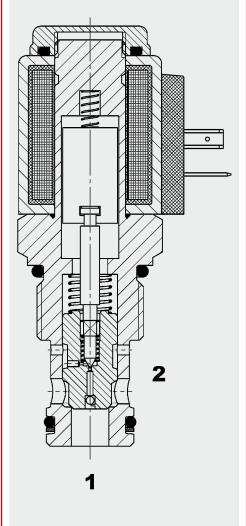
2/2 Solenoid Directional Valve UNE Poppet Type, Pilot-Operated Normally Closed (Reverse Flow) SAE-12 Cartridge – 350 bar
