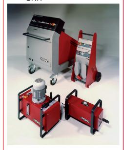
HYDAC nitrogen charging units facilitate fast and cost-effective charging or testing of the required pre-charge pressures in bladder, diaphragm and piston accumulators. They guarantee optimum use of standard nitrogen bottles up to a residual pressure of 20 bar and a maximum accumulator charging pressure of 350 bar. Portable, mobile and stationary types of N<sub>2</sub>-Server are available.
