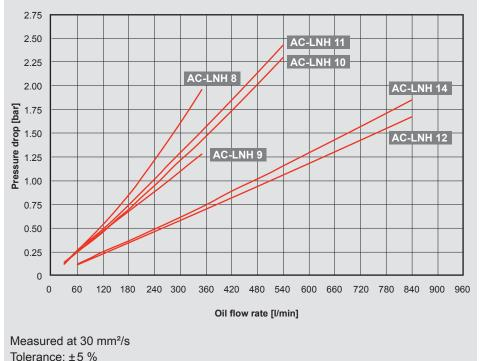
For other viscosities, the pressure drop must be multiplied by the conversion factor K:
