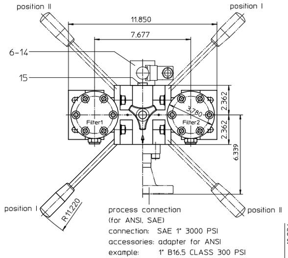
1) Connection for the potential equalisation at inlet and outlet, only for application in the explosive area.
