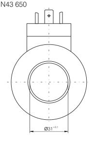
This type of coils are used for Directional control valves CETOP5.
