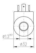
Warning: When solenoid valve should be fitted in a circuit fed by AC power a rectifier and a RAC coil must be used.
