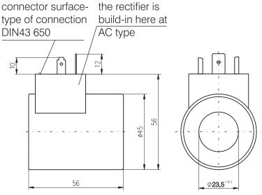
AC and DC coils have one and the same dimensions, connections and characteristics for all of type ELM-06-F-..., and one and the same for all of the type ELM-10-F-....
