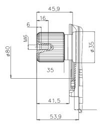
Mounting Flange C4 SAE J744 - Flange SAE C - 4 Bolts
