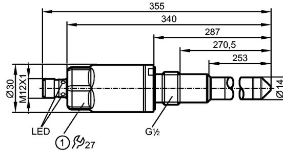
1: tightening torque 20...25 Nm
