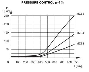
The curves have been obtained with working lines closed (without flow).
