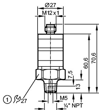
1: tightening torque 25 Nm
